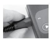
To use a light gate to control the start and stop of the stopwatch, connect a light gate to input 'A' and a light gate to input 'B'. An object passing through each light gate will start and stop the stopwatch respectively. You can also use a single light gate to start or stop a timing event and use the facia buttons to stop, reset or start depending on the input used.
