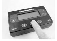
Switch on Time Machine and select 'Acceleration' followed by the input the light gate is connected to.
